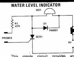
provides simple circuit This audible warning of the liquid level the probes a
